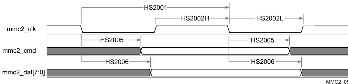
**Figure 7-78. eMMC in - HS200 SDR - Transmitter Mode**
