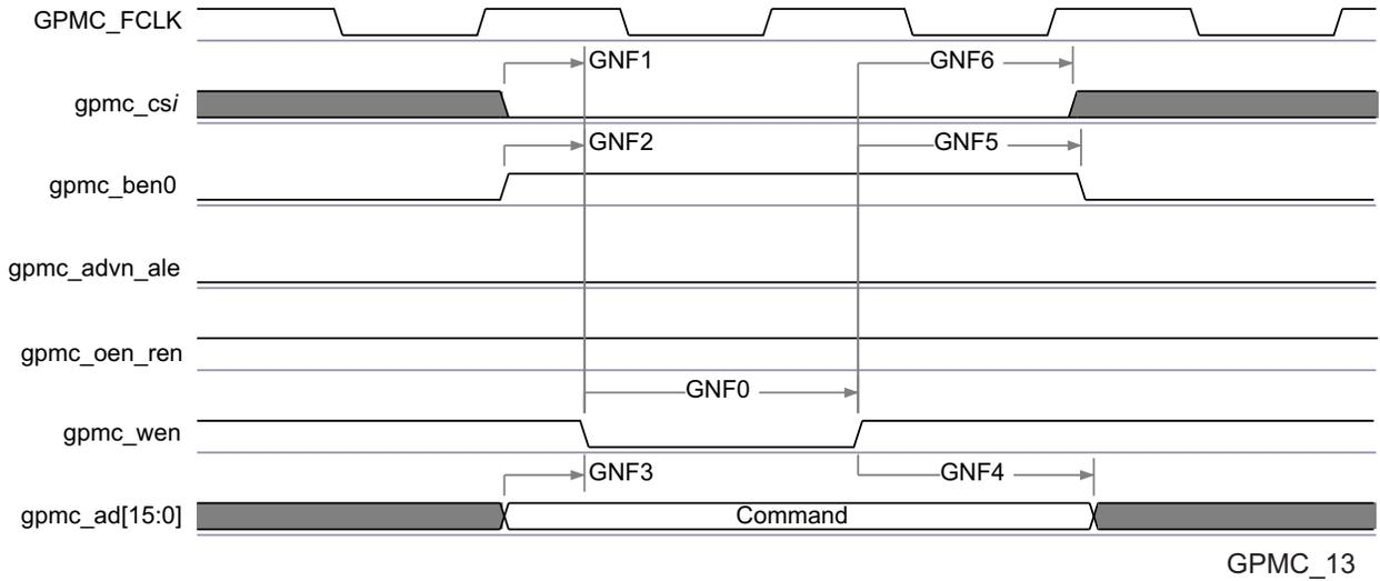
**Figure 7-19. GPMC / NAND Flash - Command Latch Cycle Timing<sup>(1)</sup>**
