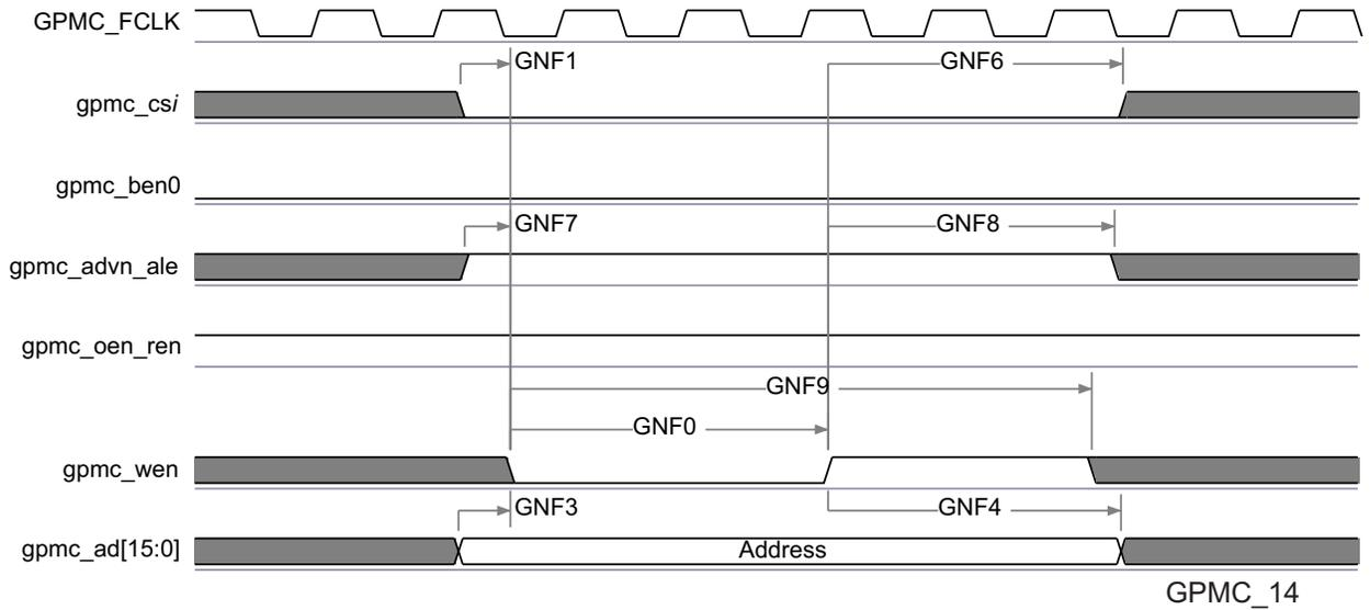
**Figure 7-20. GPMC / NAND Flash - Address Latch Cycle Timing<sup>(1)</sup>**
