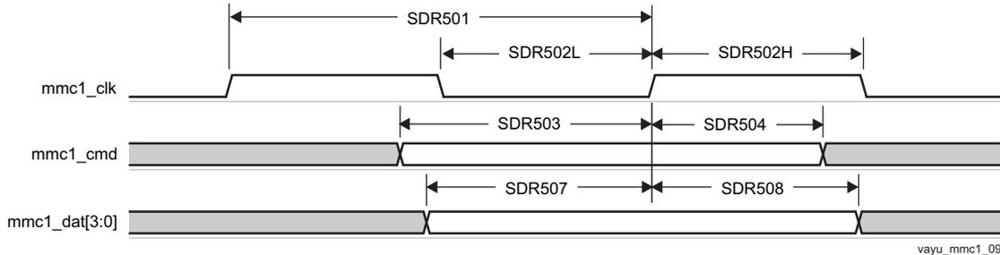
**Figure 7-68. MMC/SD/SDIO in - High Speed SDR50 - Receiver Mode**
