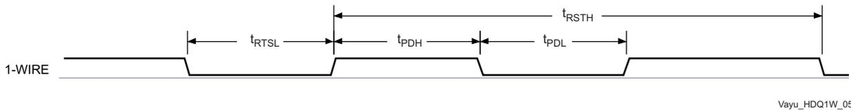
Figure 7-29. 1-Wire—Break (Reset)
