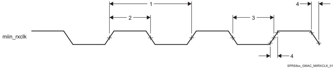
**Figure 7-51. Clock Timing (GMAC Receive) - MIIIn operation**
