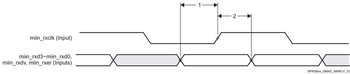
Figure 7-53. GMAC Receive Interface Timing MIIIn operation
