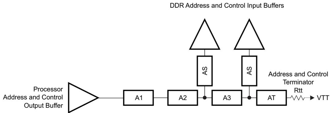
Figure 8-13. ADDR\_CTRL Topology for Two DDR3 Devices
