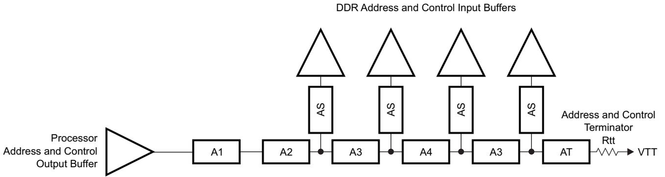
Figure 8-7. ADDR\_CTRL Topology for Four x8 DDR3 Devices
