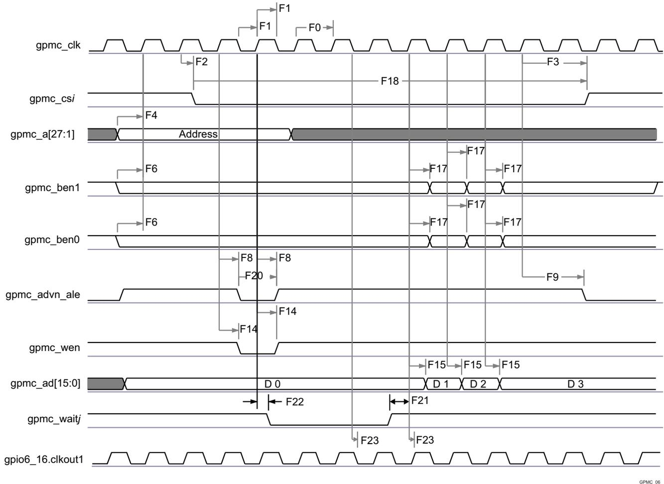
**Figure 7-12. GPMC / Nonmultiplexed 16bits NOR Flash - Synchronous Burst Write 4x16bits - (GpmcFCLKDivider = 0)<sup>(1)(2)</sup>**
