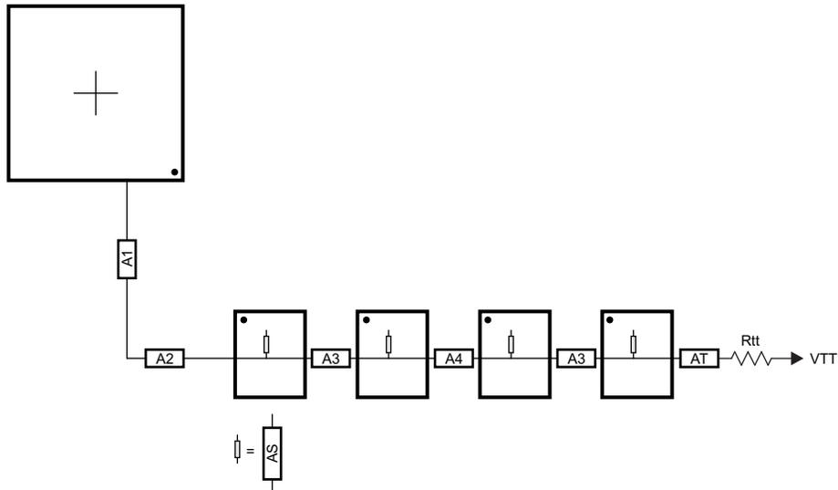
**Figure 8-9. ADDR\_CTRL Routing for Four Single-Side DDR3 Devices**
