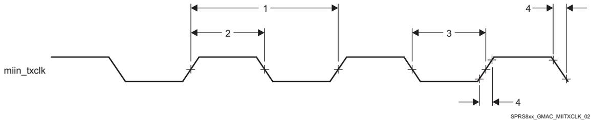
**Figure 7-52. Clock Timing (GMAC Transmit) - MIIIn operation**
