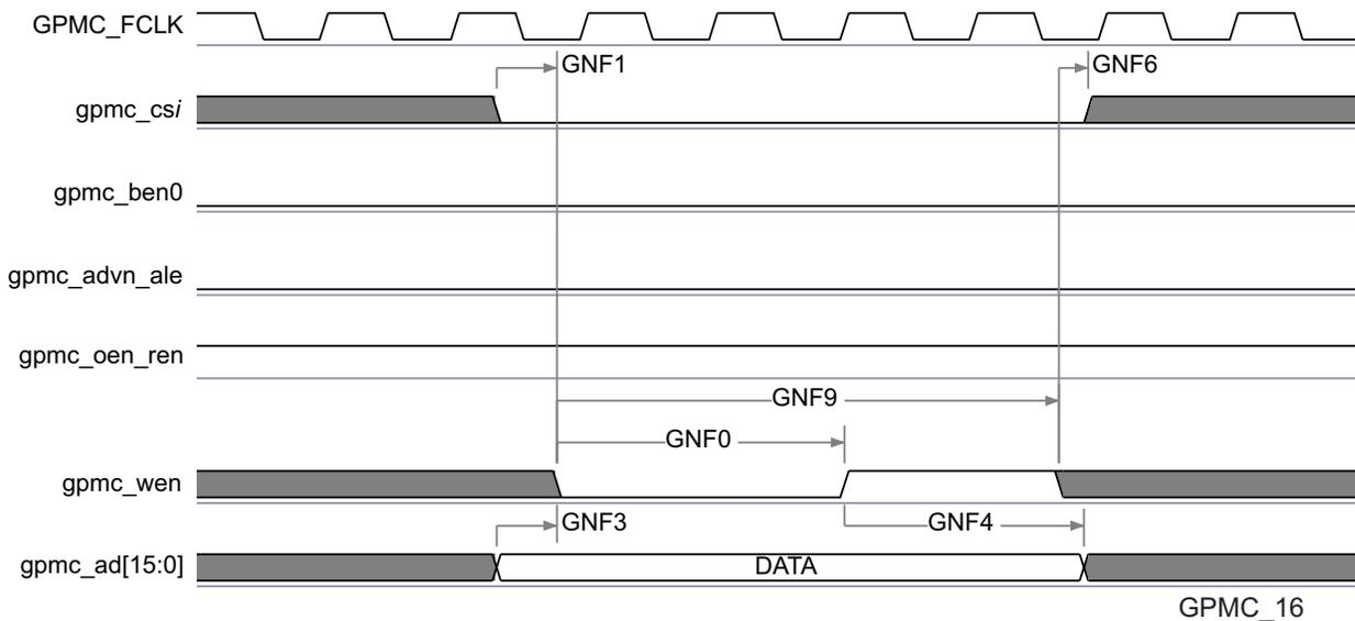
**Figure 7-22. GPMC / NAND Flash - Data Write Cycle Timing<sup>(1)</sup>**
