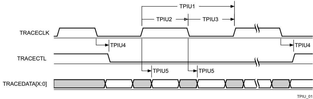
Figure 7-111. TPIU—PLL DDR Transmit Mode<sup>(1)</sup>
