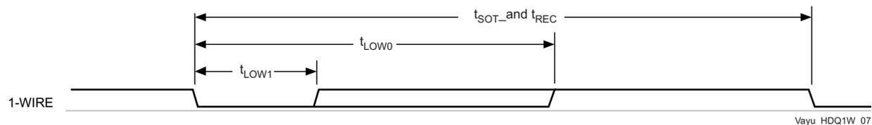
Figure 7-31. 1-Wire—Write Bit-One Timing (Command / Address or Data)
