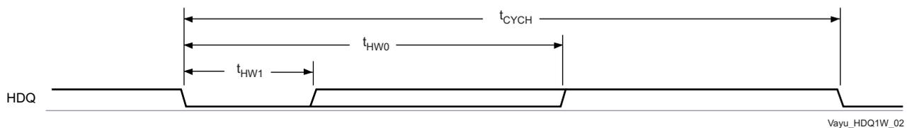
**Figure 7-26. Device HDQ Interface Bit Read Timing (Data)**
