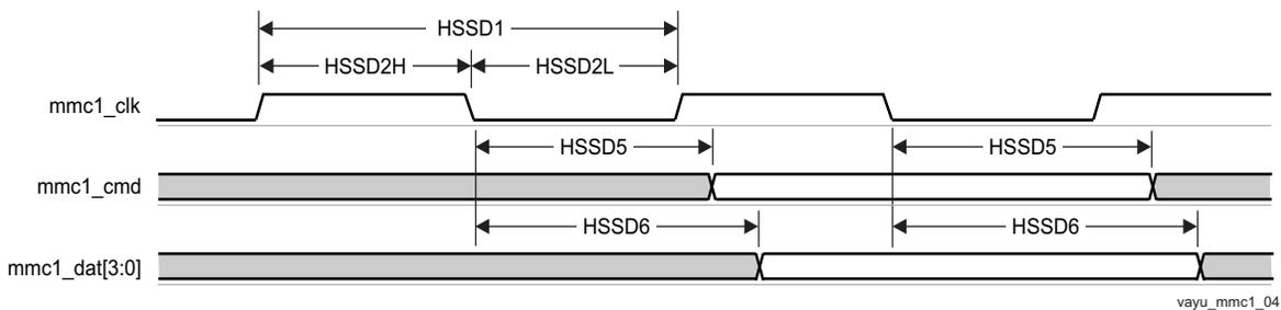
**Figure 7-63. MMC/SD/SDIO in - High Speed - Transmitter Mode**
