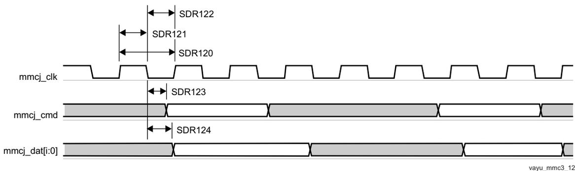
**Figure 7-86. MMC/SD/SDIOj in - SDR12 - Transmitter Mode**
