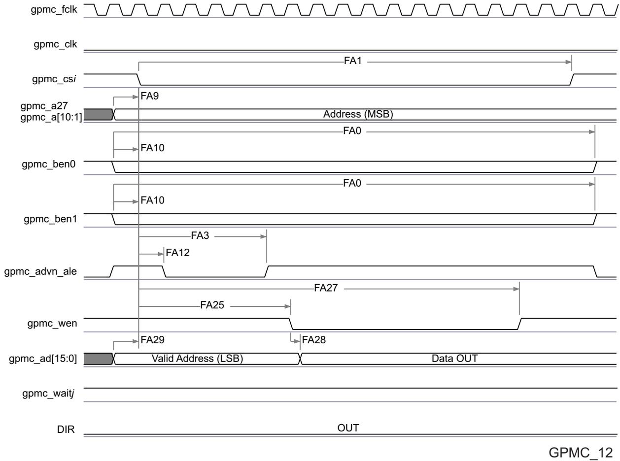
**Figure 7-18. GPMC / Multiplexed NOR Flash - Asynchronous Write - Single Word Timing<sup>(1)</sup>**
