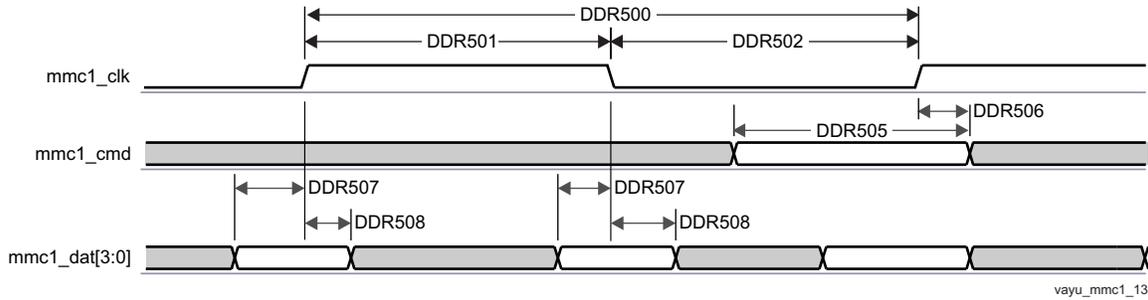
**Figure 7-72. SDMMC - High Speed SD - DDR - Data/Command Receive**
