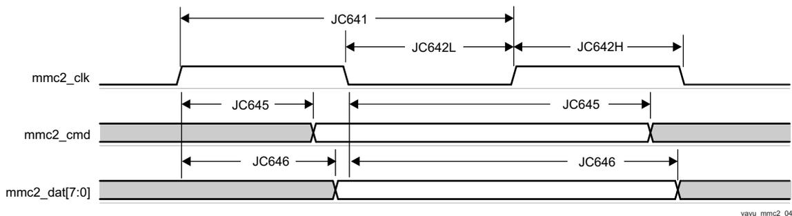
**Figure 7-77. MMC/SD/SDIO in - High Speed JC64 - Transmitter Mode**
