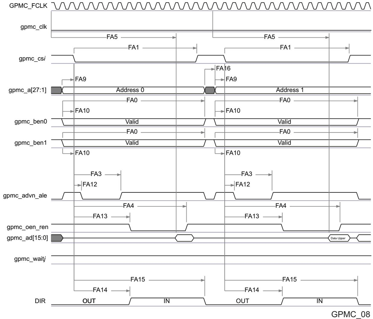
**Figure 7-14. GPMC / NOR Flash - Asynchronous Read - 32-bit Timing<sup>(1)(2)(3)</sup>**
