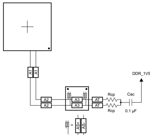
**Figure 8-16. CK Routing for Two Mirrored DDR3 Devices**
