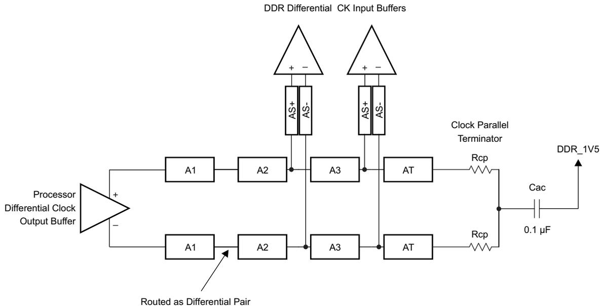
Figure 8-12. CK Topology for Two DDR3 Devices
