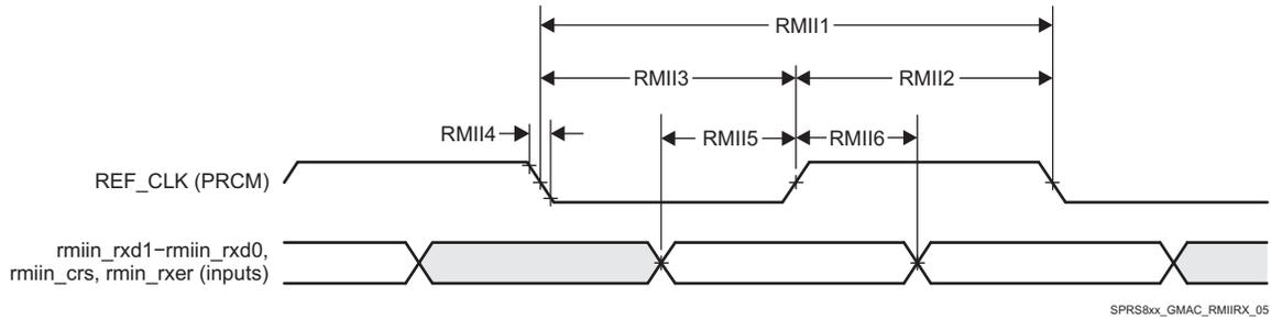
**Figure 7-56. GMAC Receive Interface Timing RMIIIn operation**
