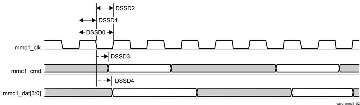
**Figure 7-61. MMC/SD/SDIO in - Default Speed - Transmitter Mode**
