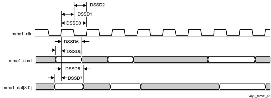
**Figure 7-60. MMC/SD/SDIO in - Default Speed - Receiver Mode**
