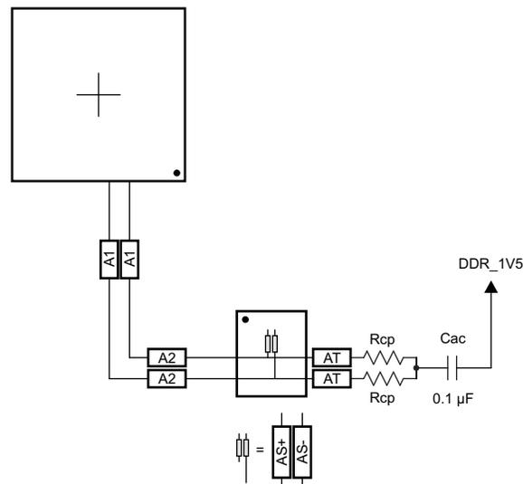
**Figure 8-20. CK Routing for One DDR3 Device**
