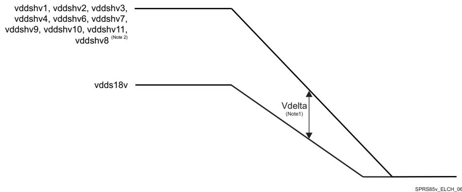
**Figure 5-4. vddshv\* Supplies Falling After vdds18v Supplies Delta**
