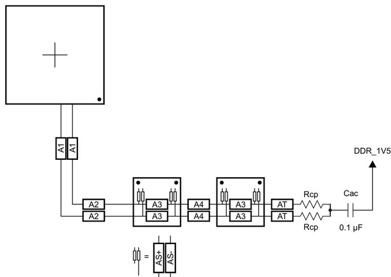
**Figure 8-10. CK Routing for Four Mirrored DDR3 Devices**
