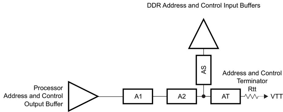
**Figure 8-19. ADDR\_CTRL Topology for One DDR3 Device**
