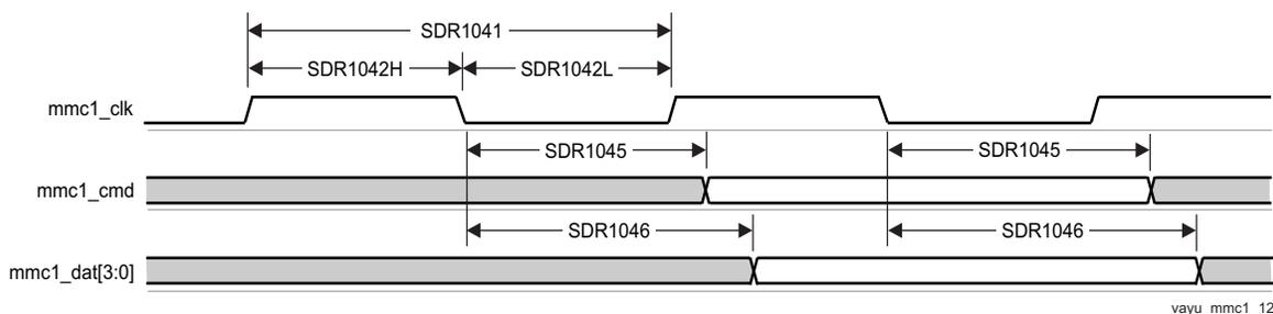
**Figure 7-71. MMC/SD/SDIO in - High Speed SDR104 - Transmitter Mode**
