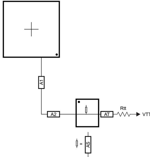
Figure 8-21. ADDR\_CTRL Routing for One DDR3 Device
