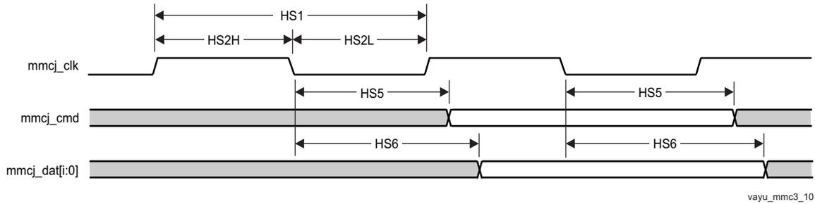
Figure 7-84. MMC/SD/SDIOj in - High Speed - Transmitter Mode
