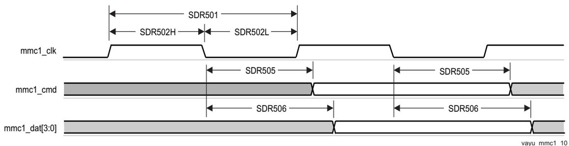
**Figure 7-69. MMC/SD/SDIO in - High Speed SDR50 - Transmitter Mode**
