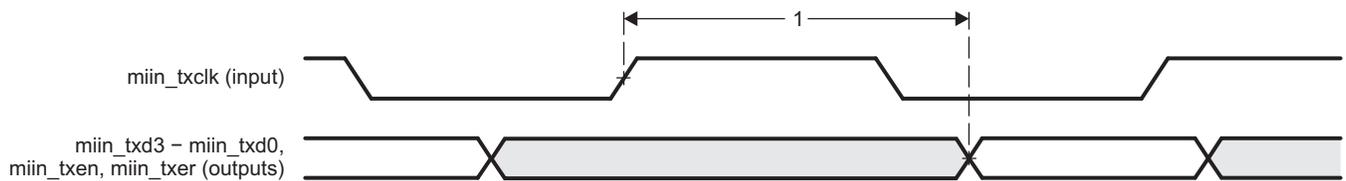
Figure 7-54. GMAC Transmit Interface Timing MIIIn operation
