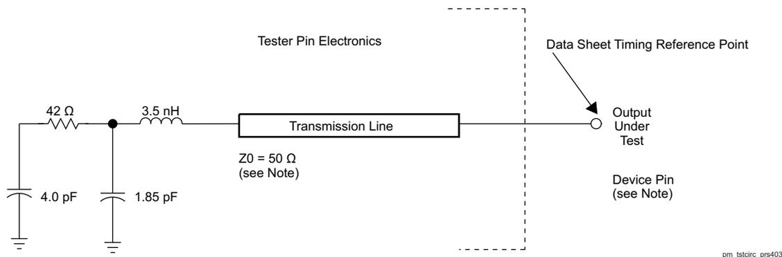
Figure 7-1. Test Load Circuit for AC Timing Measurements
