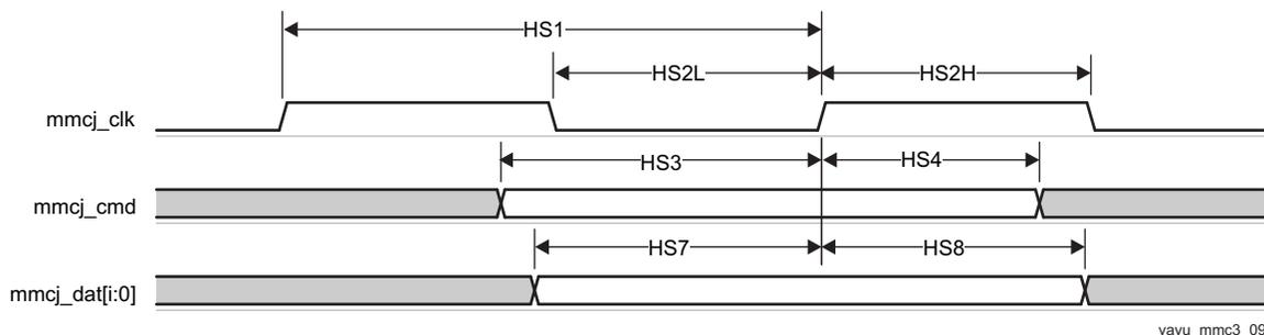
**Figure 7-83. MMC/SD/SDIOj in - High Speed - Receiver Mode**
