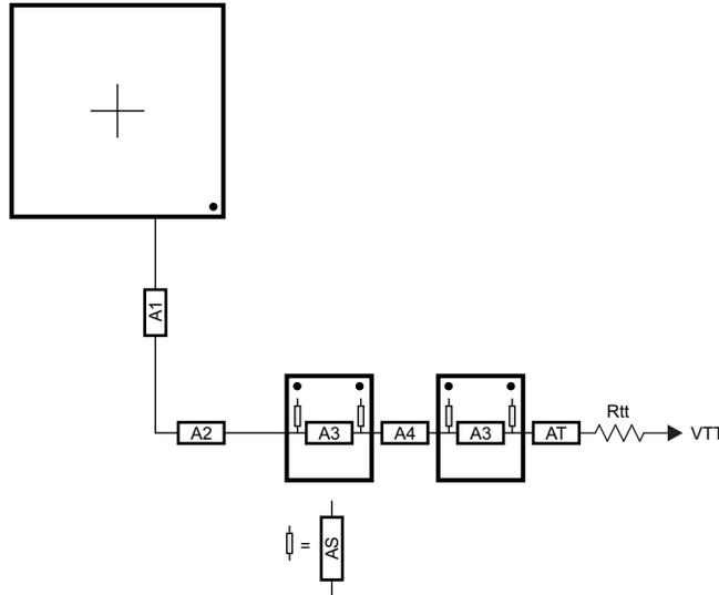
Figure 8-11. ADDR\_CTRL Routing for Four Mirrored DDR3 Devices
