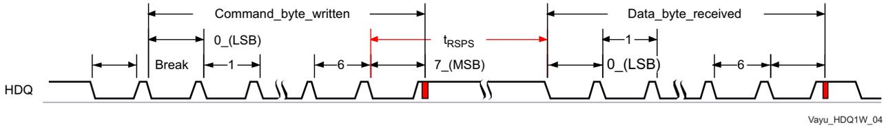
Figure 7-28. HDQ Communication Timing
