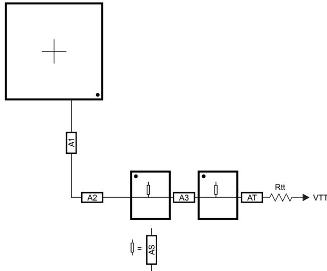
**Figure 8-15. ADDR\_CTRL Routing for Two Single-Side DDR3 Devices**
