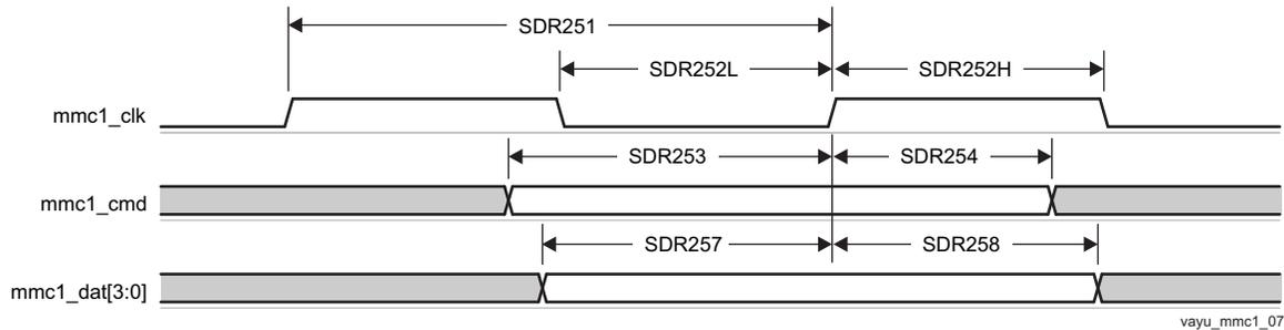
**Figure 7-66. MMC/SD/SDIO in - High Speed SDR25 - Receiver Mode**
