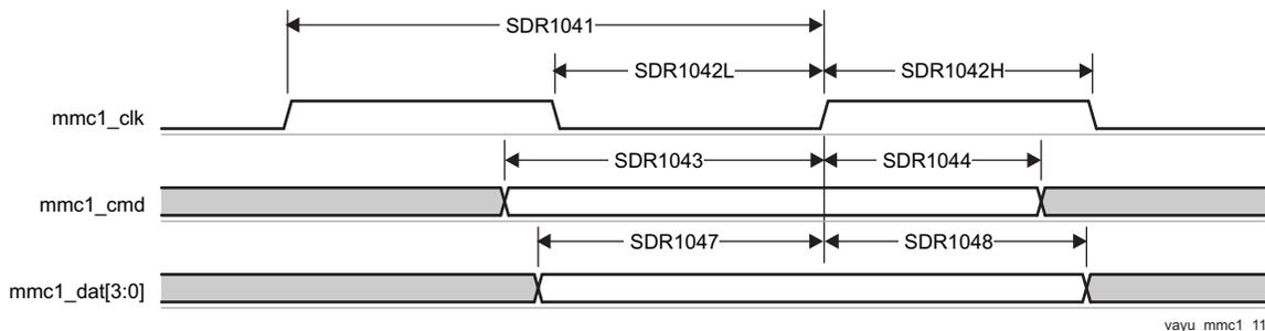
**Figure 7-70. MMC/SD/SDIO in - High Speed SDR104 - Receiver Mode**
