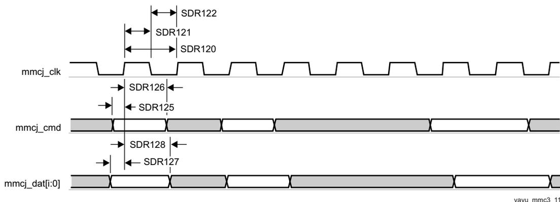
**Figure 7-85. MMC/SD/SDIOj in - SDR12 - Receiver Mode**
