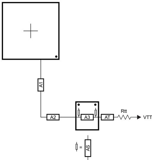
Figure 8-17. ADDR\_CTRL Routing for Two Mirrored DDR3 Devices
