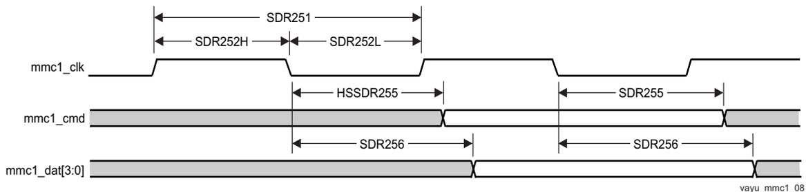
**Figure 7-67. MMC/SD/SDIO in - High Speed SDR25 - Transmitter Mode**
