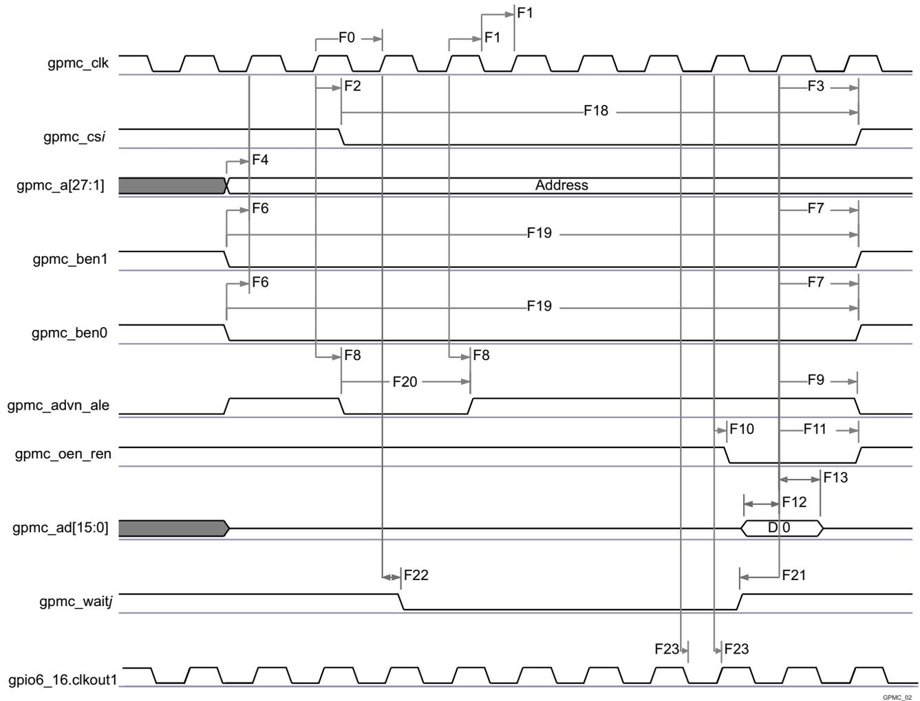
**Figure 7-8. GPMC / Nonmultiplexed 16bits NOR Flash - Synchronous Single Read - (GpmcFCLKDivider = 0)<sup>(1)(2)</sup>**
