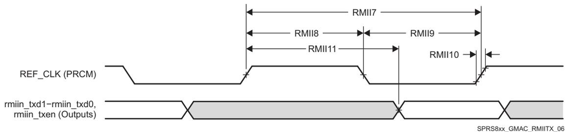
**Figure 7-57. GMAC Transmit Interface Timing RMIIIn Operation**
