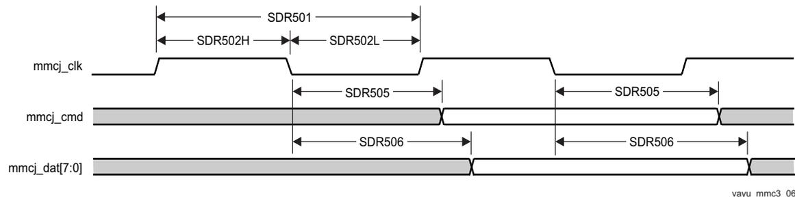
**Figure 7-90. MMC/SD/SDIOj in - High Speed SDR50 - Transmitter Mode**
