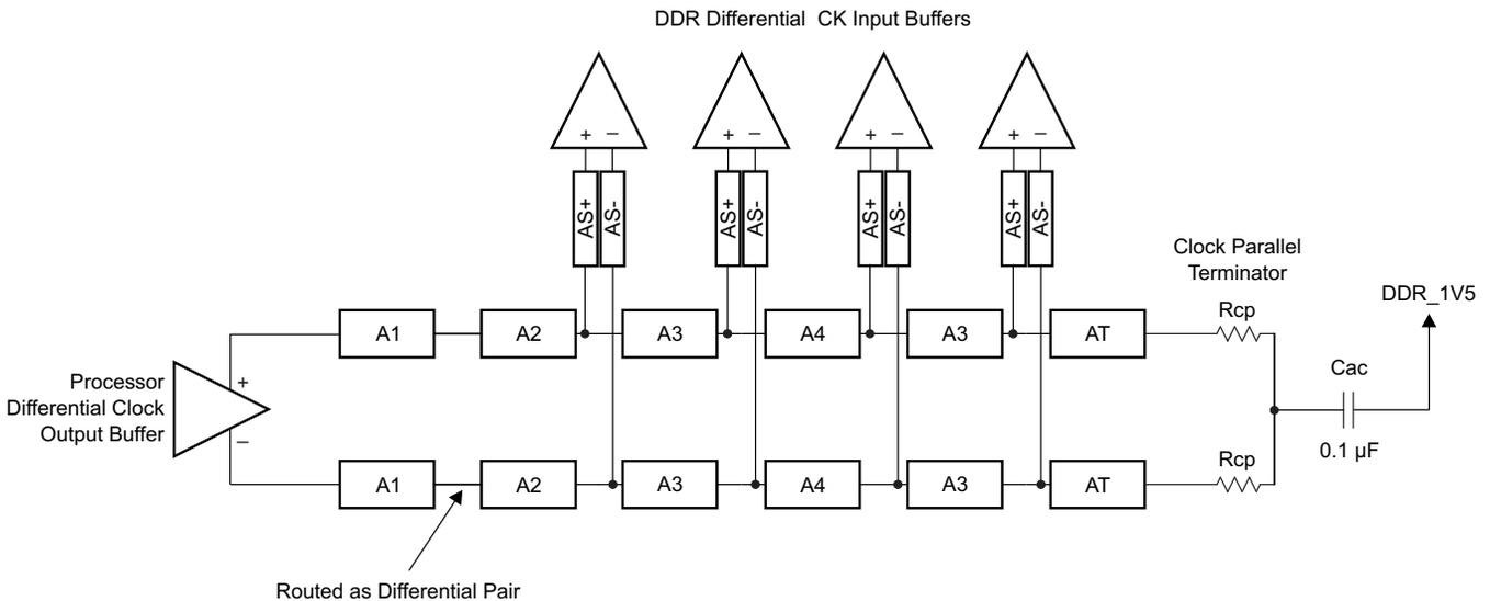
Figure 8-6. CK Topology for Four x8 DDR3 Devices
