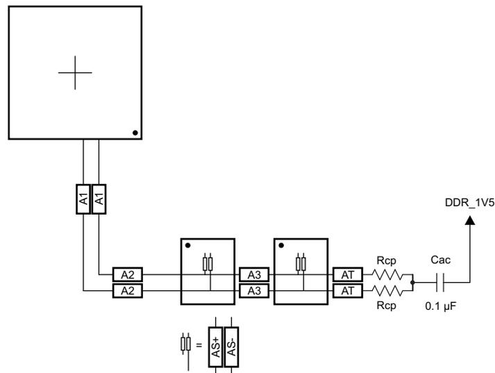
Figure 8-14. CK Routing for Two Single-Side DDR3 Devices
