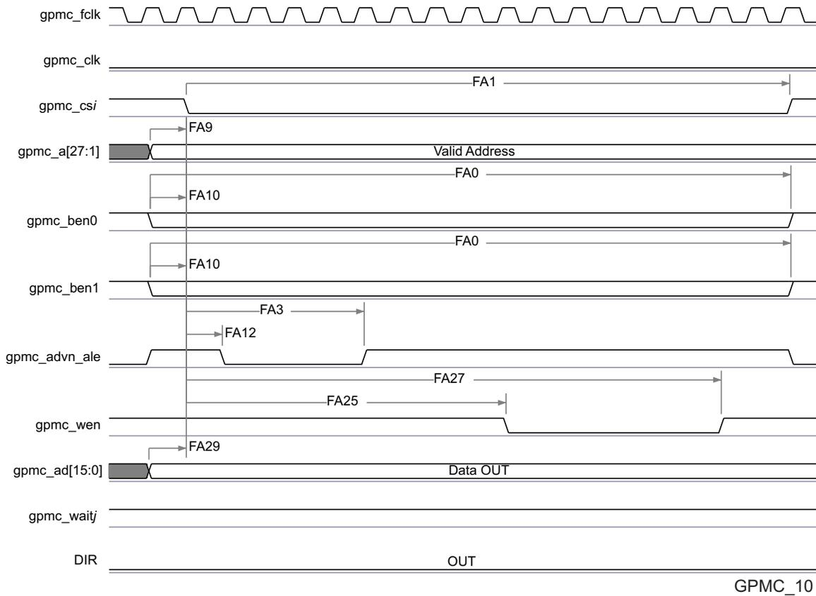
**Figure 7-16. GPMC / NOR Flash - Asynchronous Write - Single Word Timing<sup>(1)</sup>**
