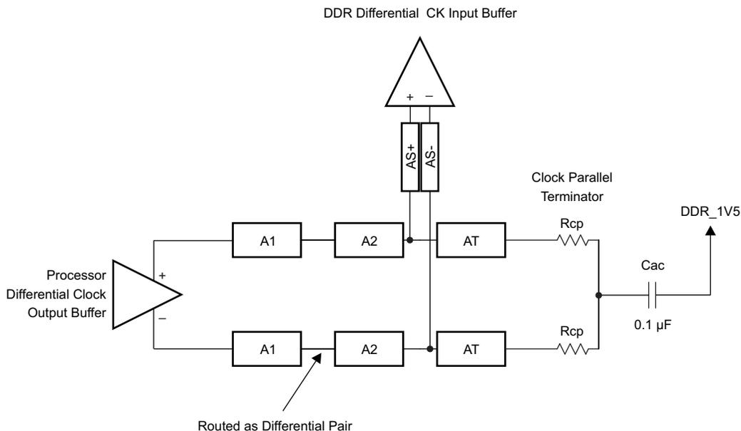
Figure 8-18. CK Topology for One DDR3 Device
