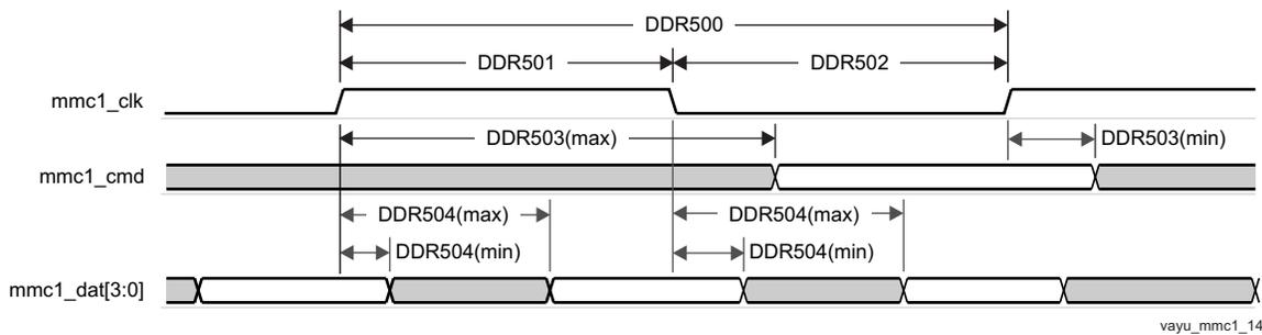
**Figure 7-73. SDMMC - High Speed SD - DDR - Data/Command Transmit**
