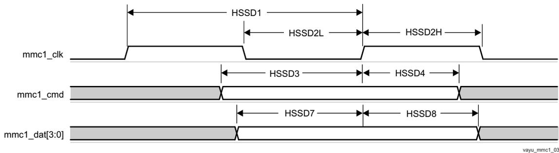
**Figure 7-62. MMC/SD/SDIO in - High Speed - Receiver Mode**
