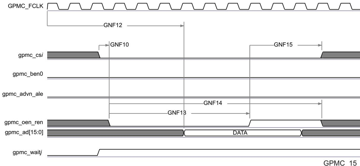
**Figure 7-21. GPMC / NAND Flash - Data Read Cycle Timing<sup>(1)(2)(3)</sup>**
