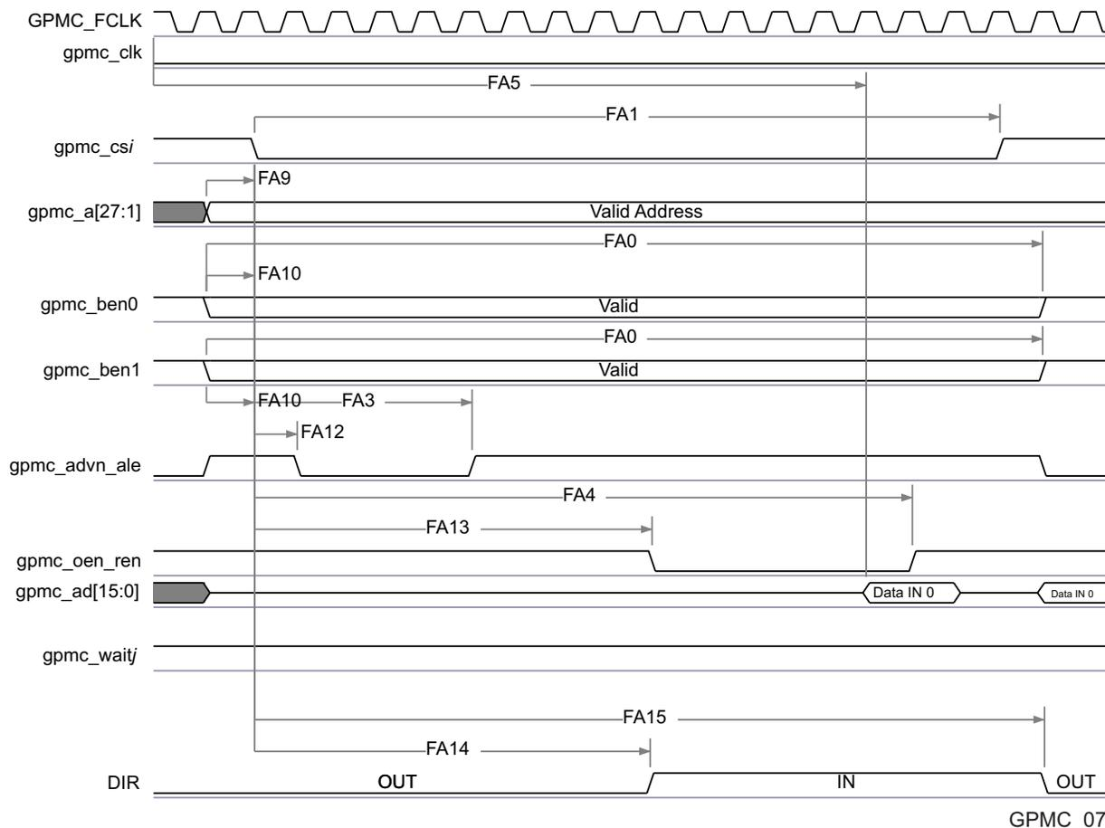
**Figure 7-13. GPMC / NOR Flash - Asynchronous Read - Single Word Timing<sup>(1)(2)(3)</sup>**
