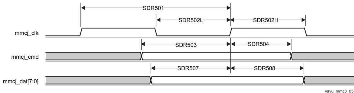
**Figure 7-89. MMC/SD/SDIOj in - High Speed SDR50 - Receiver Mode**
