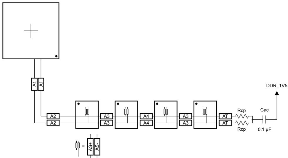
Figure 8-8. CK Routing for Four Single-Side DDR3 Devices
